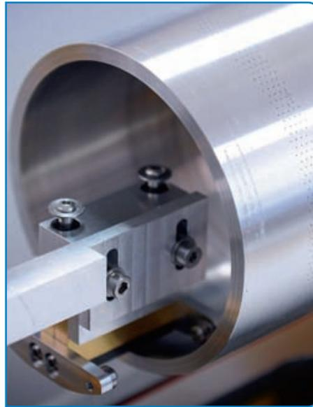
**Archipelago Powerdrop test rig showing nozzles in rotating drum dispenser**
