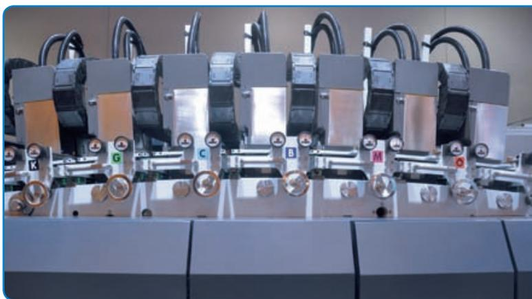
**Seven colour Kodak Stream inkjet heads mounted onto a Uteco transport to deliver flexible packaging onto foils at speeds up to 200 m/min**
